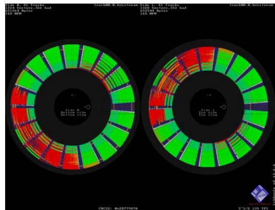
Figure 2 HxC floppy disk track analyzer. Red parts indicate sectors with errors.
