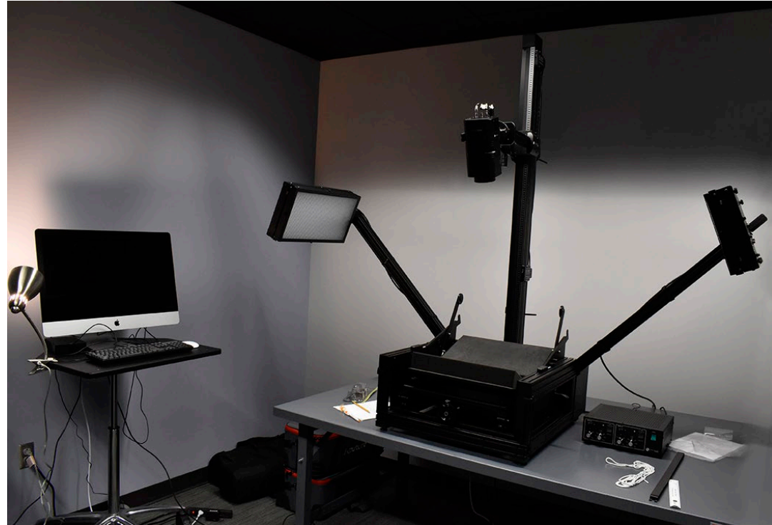
DT Atom is used to image rare / fragile materials not suitable for a flatbed scanner.
