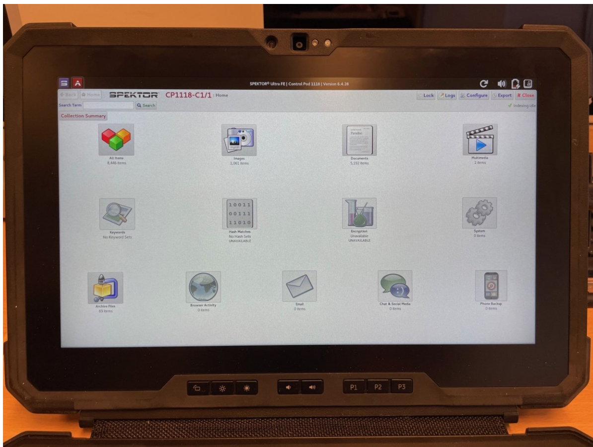
SPEKTOR Ultra Digital Forensics machine in Collector Mode for rapid appraisal
