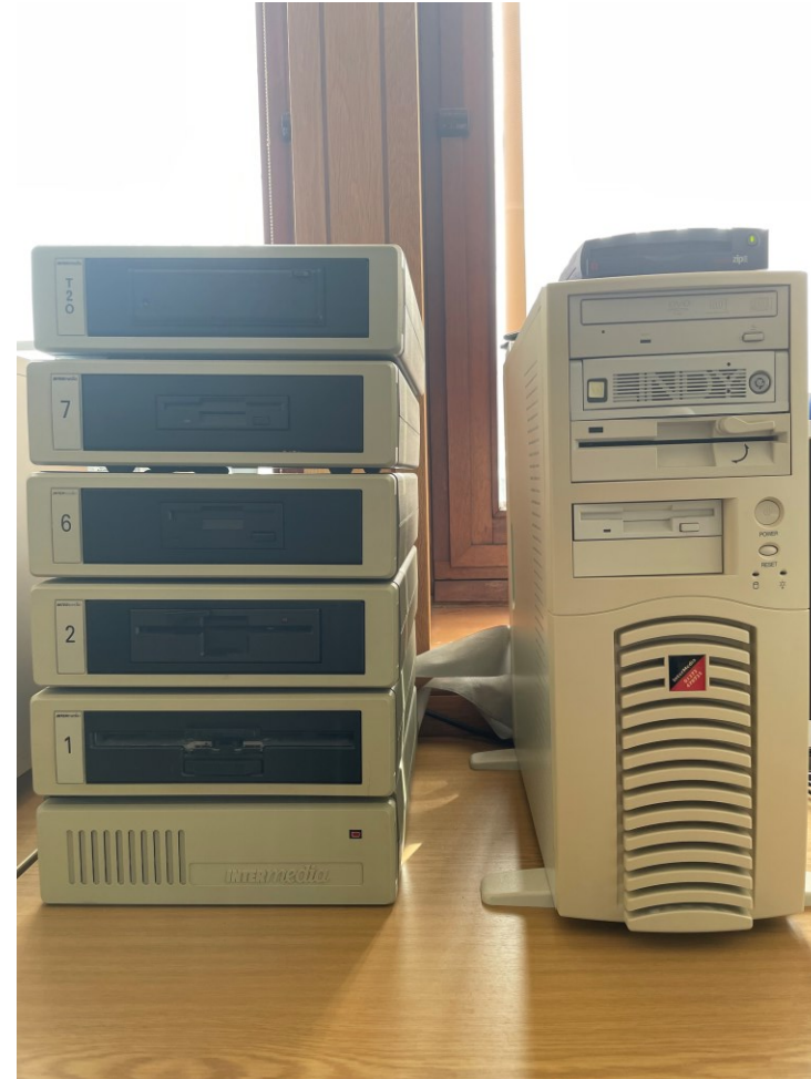
Intermedia and Windows XP machine used for non-forensic data extraction from other magnetic media
