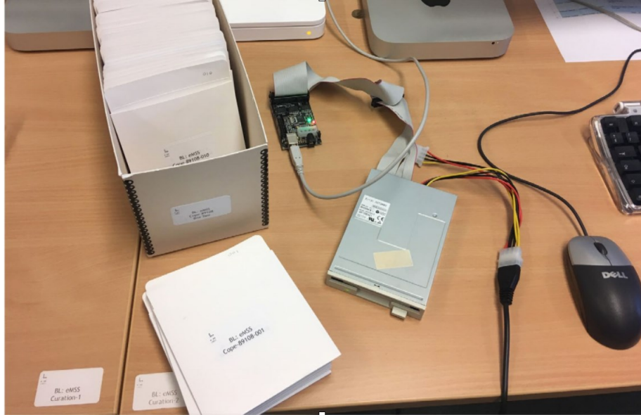
Kryoflux creating bit-level captures of 3.5inch floppy disks from the Wendy Cope Archive (Add MS 89108)
